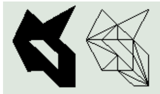
Figure 15.2 Output from TriangulatorTest : The surface generated rendered both as a solid (left) and as a wireframe (right)
